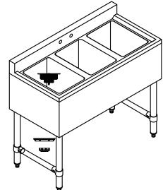
3.Put the rubber washer under the stainer body, insert them inside of the sink drain hole. Under the sink bowl, connect the paper gasket and lock nut to the stainer body in turn and tighten.
