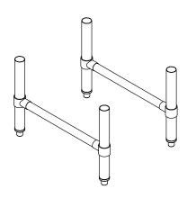
1.Insert the leg brace into leg brace connectors, fix the leg brace with screws. Insert the legs through leg brace connectors at same level, fix the legs with screws, "H" shape legs are assembled.
