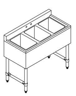
2.Turn over the main body of barsink on the floor, insert the "H" shape legs into the sockets under the bar sink with 8\*1\*10 screws, tighten the screws, stand up the Bar sink
