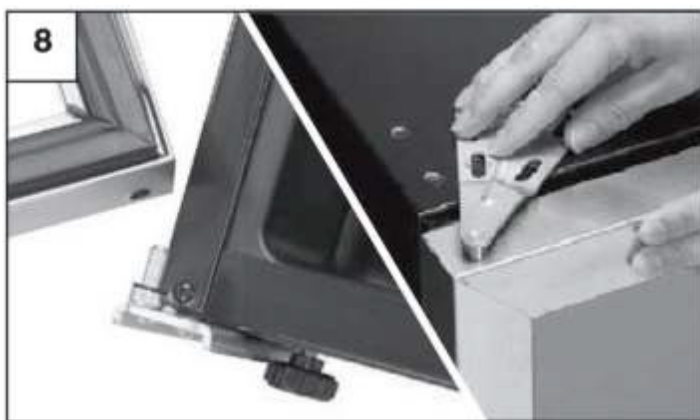
8. To reattach the door, place the door onto the bottom axle insert. Place the top bracket into the door and align the metal bracket holes over the holes in the top of the unit cabinet. Tighten the three screws to hold in place.
