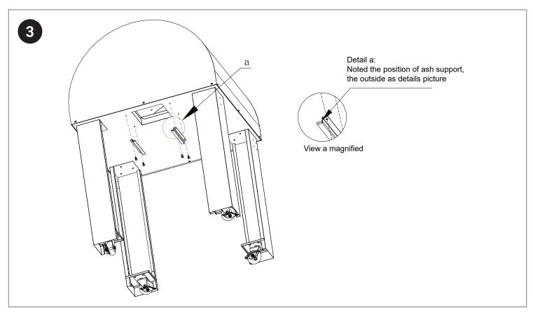
\* The ash support holds the ash box, enabling easy cleanup after cooking.
