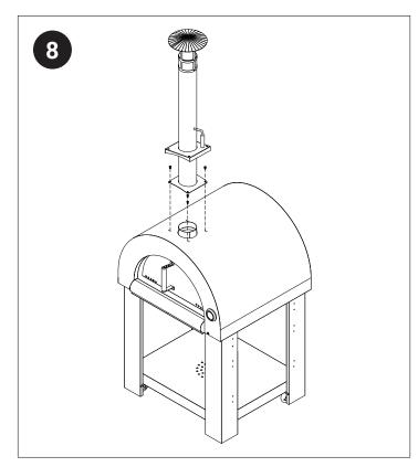
\* The chimney cap plays a key role in directing smoke away from the oven and controlling draft.
