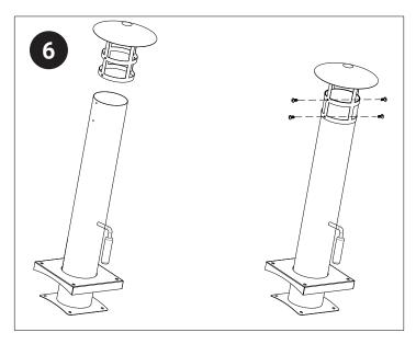
The chimney cap plays a key role in directing smoke away from the oven and controlling draft.
