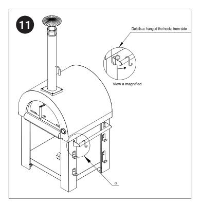
\* These hooks provide additional storage space and easy access to your cooking utensils while using the oven.
