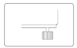
(which are optional). To stabilize the unit, rotate these feet clockwise. This downward extension ensures that the refrigerator remains steady and well-grounded during daily operations.
