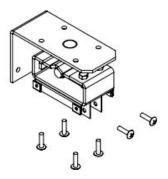
Step 2: Mount the L-Bracket hinge. Insert two 1/4-20-1" screws, and attach it to the left side.
