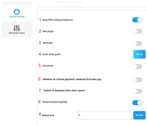
**Quick setup guide:** Enabling this function grants access to a quick setup page containing multiple commonly used setup menus for debugging engineer.
