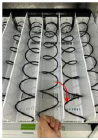
Comparison of spiral in default position and pull-out position.
