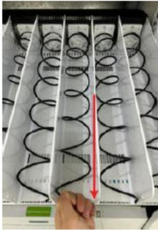
Rotate the spiral to the desired position. Release the spiral.
