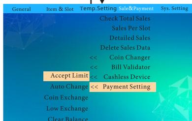
When the low value of no change is set to 0, even if the machine has no change, the machine purchase interface will not prompt "insufficient change". When the machine prompts that the change is insufficient, the purchase of goods needs to be invested in coins equal to the price of goods. Otherwise, it may not give the change after the purchase of goods.
