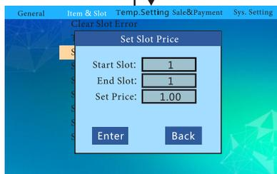
Press the digital keyboard to input the initial cargo lane number and ending cargo lane number to be set, and set the selected cargo lane number price. Press "Enter" to save the setting.
