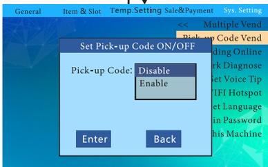
Press ▲ 2 / ▼ 8 in the keyboard to select to disable or enable the pick-up code switch, press the "Enter" button to save the settings.
