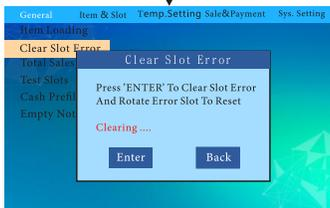
When the cargo lane failure is cleared, the faulty cargo lane spring will rotate one full turn back to the initial position (reset)
