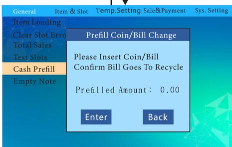
Check whether the change amount of the input is consistent with the current prefill amount displayed. Confirm that there is no mistake and press the "Enter" button.
