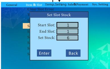
Press the digital keyboard to input the initial cargo lane number and ending cargo lane number to be set, and set the existing number of the selected cargo lane number. Press "Enter" to save the setting (the existing number must be consistent with the actual number of goods in the cargo lane)
