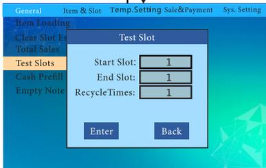
Input the starting cargo lane number and ending cargo lane number, and set the number of cycle tests (turn off the optical inspection before testing the cargo lane or block the optical inspection by hand when the cargo lane rotates, otherwise the spring can not be reset)
