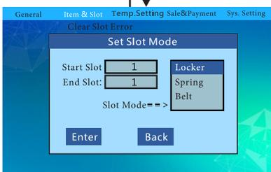
Press the digital keyboard to input the initial cargo lane number and ending cargo lane number to be set, and set the driving mode of the selected cargo lane. Press "Enter" to save the setting.
