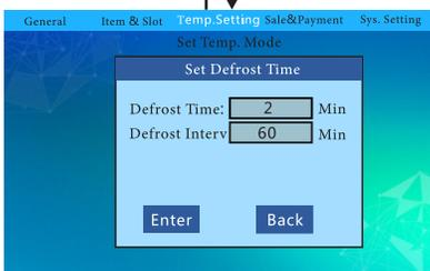
Set the defrosting time and downtime defrosting cycle (defrosting time interval), press the "Enter" button to save the settings.
