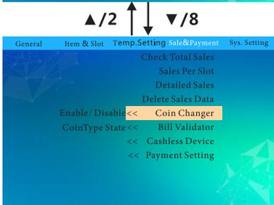
Press ▲2/▼8 to select to disable or enable coin change. If the machine needs coin change, the coin change switch must be turned on. Press "Enter" to save the settings.
