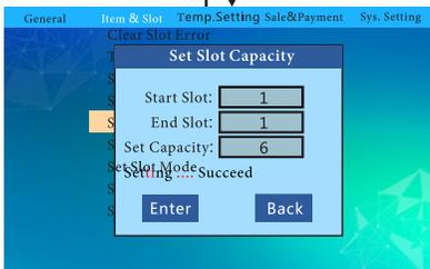
Press the digital keyboard to input the initial cargo lane number and ending cargo lane number to be set, and set the maximum capacity of the selected cargo lane. Press "Enter" to save the setting.
