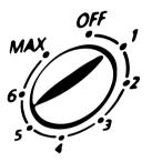
To adjust the temperature turn the knob clockwise. The higher the number the lower the temperature. Generally, position '4' or '5' is suggested to make a normal setting. The "OFF" position will stop the compressor while the "MAX" position will allow the compressor to continually run Do not keep the knob at this point for more than 4-5 hours
